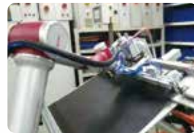
Window blinds riveting
