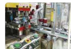
Ball-bearing press fitting machine loading
