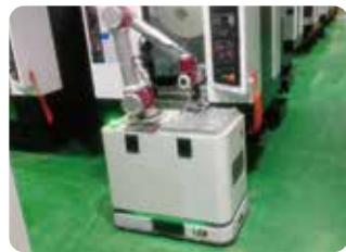
Hybrid robot CNC machine loading
