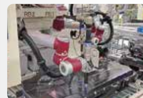
Battery residue removal
