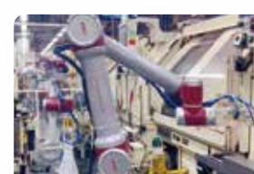
Transmission parts machine loading
